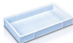
RB318304: 22 litres Solid 30"x18" confectionery tray Ext: 762 x 457 x 92mm Int: 715 x 412 x 72mm Wt: 1.8 Kg, colour: natural Compatible with lid ref. LI301804 and dolly ref. DO301801
